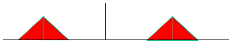
Figure.1 : Spectrum of the DSBSC wave
