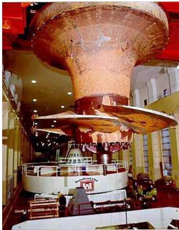
Figure 30.1 A typical Kaplan Turbine
