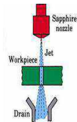
Mechanism of material removal: Erosion
