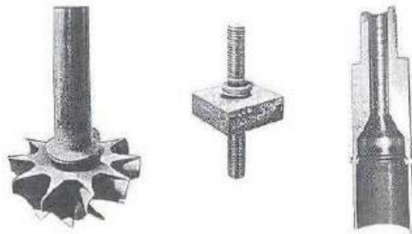
FIGURE 36-6 Some typical friction-welded parts. (Left) Impeller made by joining a chrome-moly steel shaft to a nickel-steel casting. (Center) Stud plate with two mild steel studs joined to a square plate. (Right) Tube component where a turned segment is joined to medium-carbon steel tubing. (Courtesy of Newcor Bay City, Div. of Newcor, Inc.)
